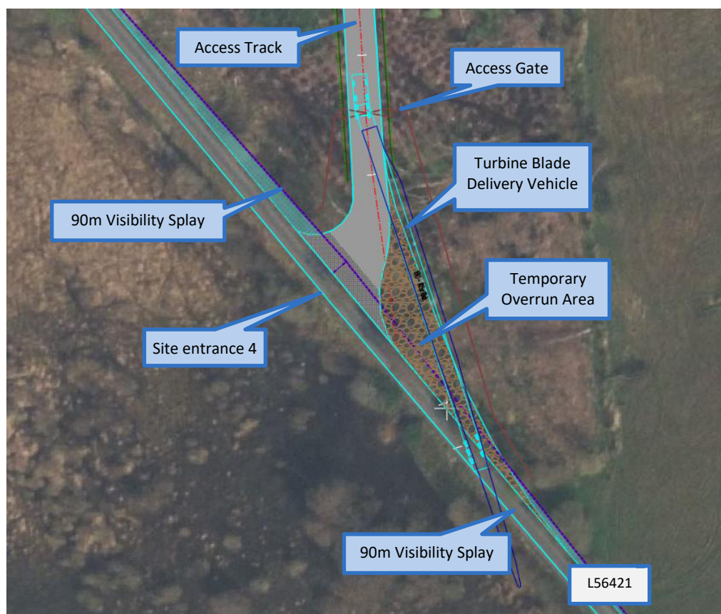
Figure 10 – Site Entrance 4 on the L56421
